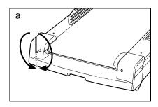
b. If the walking belt slips when walked on, first remove the key and UNPLUG THE POWER CORD. Using the allen wrench, turn both rear roller bolts clockwise 1/4 of a turn. When the walking belt is correctly tightened, you should be able to lift each side of the walking belt 3 to 4 inches off the walking platform. Be careful to keep the walking belt centered. Plug in the power cord, insert the key and carefully walk on
